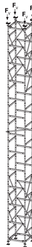
8.29 m – 12.29 m: 3 diagonal braces at the top and bottom. Plus horizontal cross strut at H/2 .
