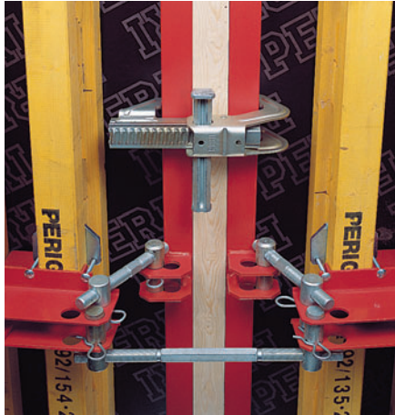
Adjusting Spindles 500 positioned in the T-waler and secured by means of Cotter Pins 5/1.
